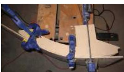
Each side of the cab will have one of the ribs (made of pine or harder wood) connected to it with threaded inserts. The main stress will be downward and the vertical inserts will take the load off the few horizontal ones I use (like these). You can also see on this picture the idea behind the curved skeleton. It will continue in a 2nd piece that will curve along the back to the bottom so that what I end up with is a nice curve outlining the cab...no squares here.
