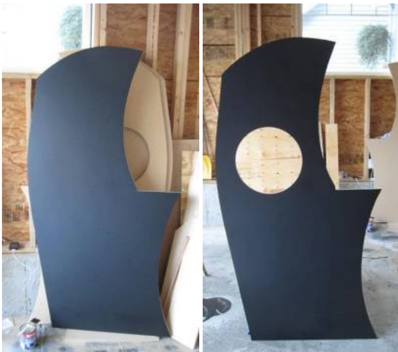
I then laminated the inside which you can see is a patchwork of odds and ends. I put as much towards the center as I could because I will be mounting strips and don't want parts of the strip on laminate and part off:
