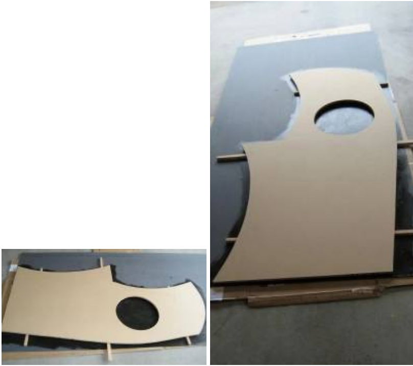
Here is the outside of side 1 fully laminated before and after side hole was trimmed:
