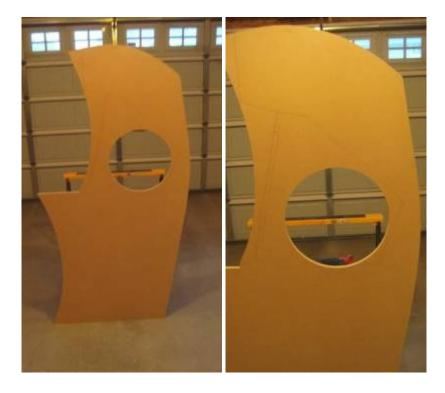
I cut a slot into the center of the hole as I will be running the T-Molding around the hole like I have seen on a few other cabs. I think it will look pretty good when done with the green neon light and artwork and T Molding as a trim:
