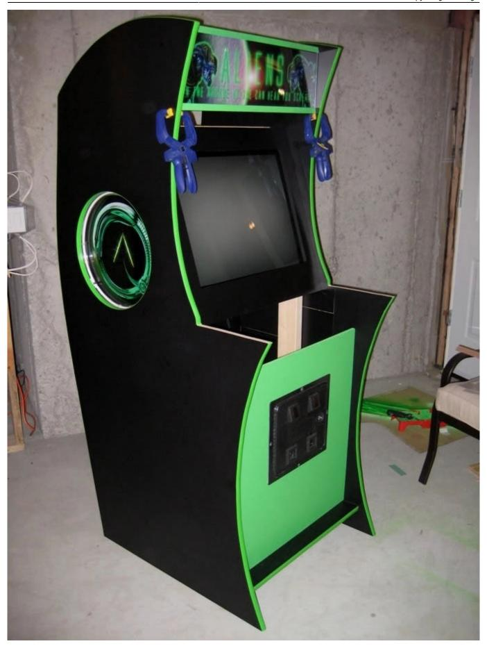
I use Lepage's blue contact cement from Home Depot to laminate the cabinet...it looks like the alien slop but spreads on super easy with a disposable paint brush. It also dries quickly but not too quickly...in other words it gives you enough time to apply glue on both sides before joining (15 to 20 mins).
